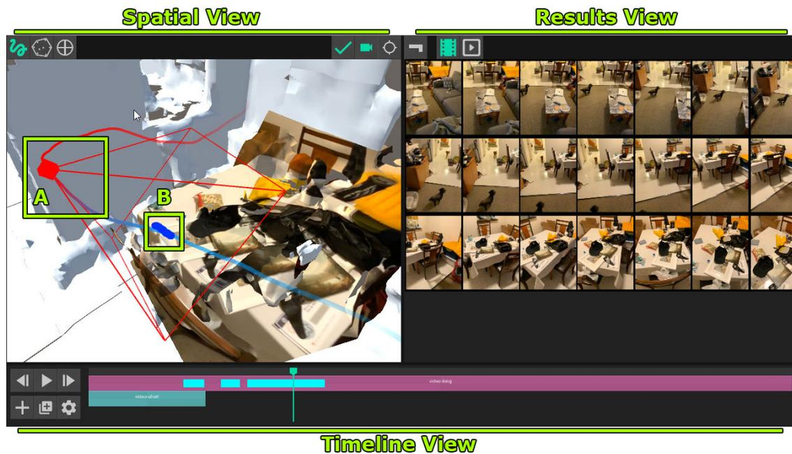
Fig. 2. AR-Video Query interface. Top left shows the spatial view, top right show the results view, and bottom shows the temporal timeline view. Callout A shows the camera position rendered in the spatial view. Callout B shows an example paint stroke query.
