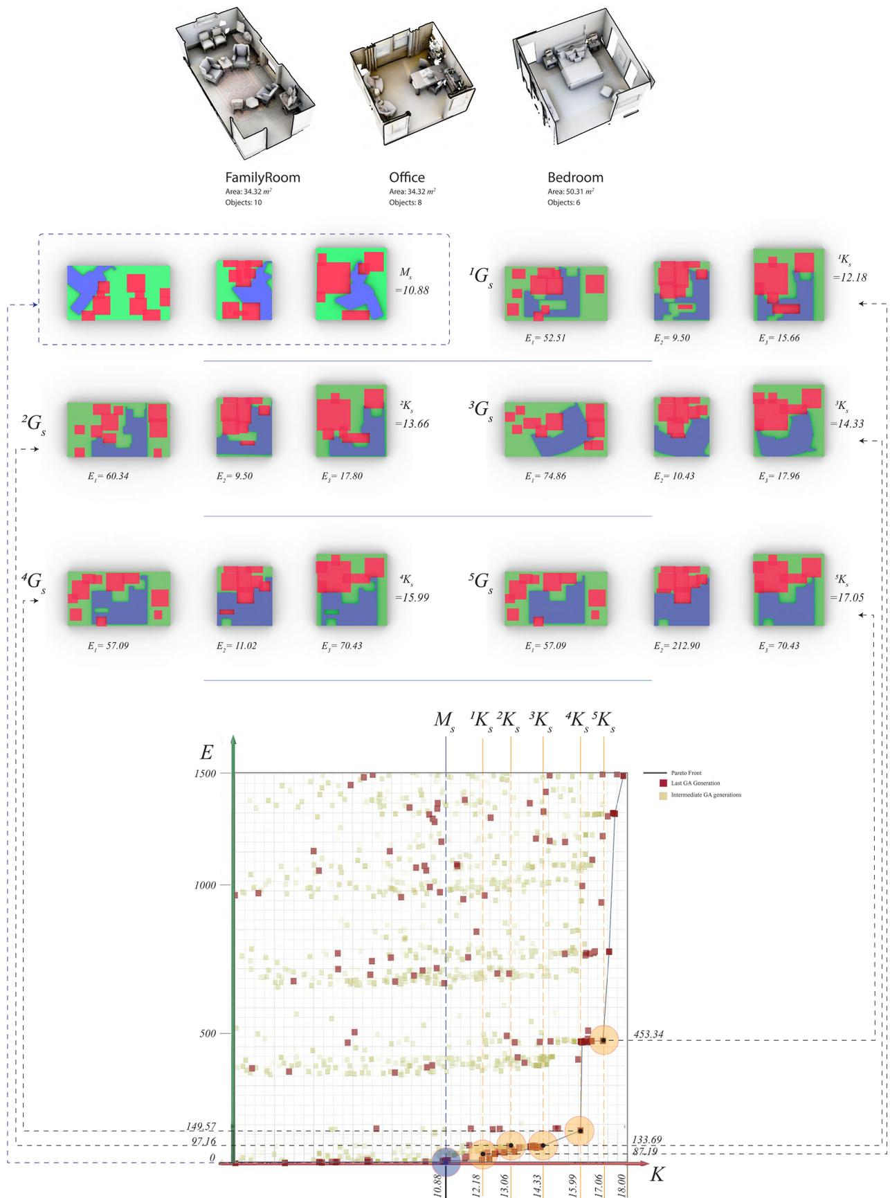
Figure 5: Furniture optimization and manipulation. In each step, a 10% increase of mutual space area ( $K$ ) is determined, while minimizing the overall effort needed ( $E$ ) for the required transformation ( $G$ ).
